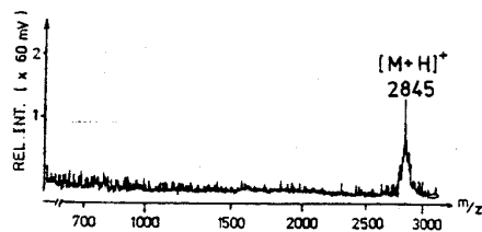
Fig. 7. Matrix-LD spectra of mellitin/NicAc accumulated from 12 single laser shots.
